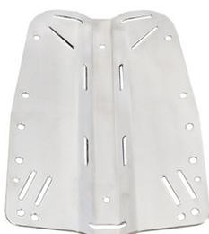
Stainless-steel backplate made of salt water resistant stainless-steel. Edges bevelled on a NC cutter, manually polished for perfect flattening of sharp edges, which could dilacerate the strap.
