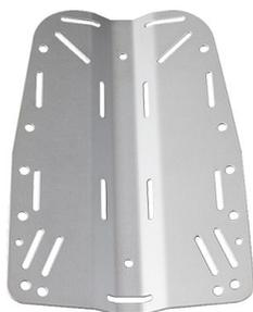
Dural backplate made of aluminium alloy resistant to salt water. Backplate is hard anodized. Edges bevelled on a NC cutter. Thanks to low weight of 0.8 kg it is ideal for travelling by plane.
