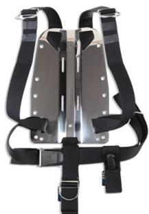
Dural backplate, thickness 3 mm with PA harness, stainless-steel D-rings and stoppers, stainless-steel buckle, crotch strap, buoy pocket and pocket with knife. Backplate is made of aluminium alloy resistant to salt water. Backplate is hard anodized. Edges bevelled on a NC cutter.
