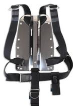
Small sized backplate to fit smaller backs, 5 cm shorter than our normal backplates. Fits together with our KIDDO wing and also with all other wing types. Stainless-steel backplate, thickness 3 mm, made of salt water resistant stainless-steel with edges bevelled on a NC cutter, manually polished for perfect flattening of sharp edges.
